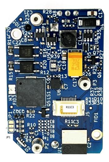
Connector: **R11C3** for future expansion boards of the lock electronics
