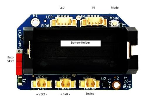
Connector: **LED** 3 separate LEDs or RGB LED
